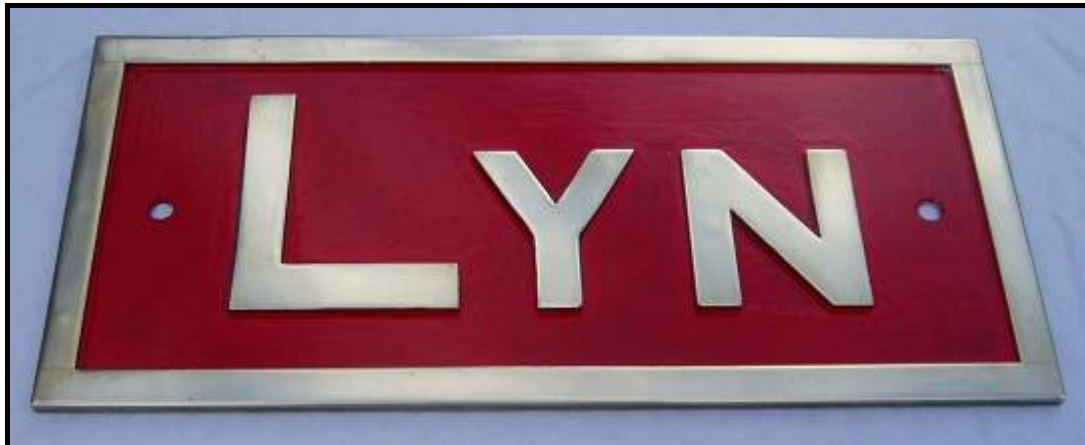
'Lyn' nameplate made by Peter Miles in the original style with riveted brass plate construction, one of a pair to be fitted to the locomotive.
