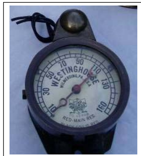
Westinghouse brake air gauge (right) and steam chest pressure gauge (below)
